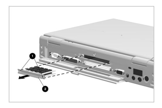
Figure 5-18. Removing a Memory Module
